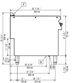
EQ = Equipotential screwG = Gas connection
